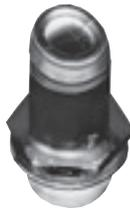
Connector seat and/or threads at top of shielding barrel badly nicked or corroded. Terminal barrel sleeve cracked.
