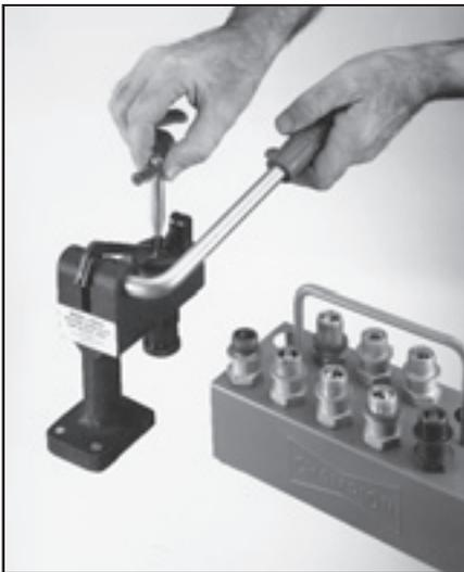
Since the Champion Model 2500A gap-setting tool adjusts two electrodes simultaneously, it is particularly useful for high-volume gap-setting requirements. This tool easily adjusts four-electrode N Type and two-electrode E Type aviation spark plugs.
