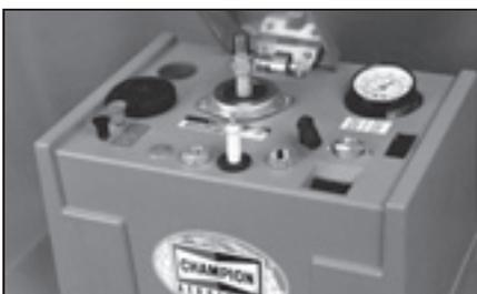
Cleaning barrel end with Model CT-475AV Cleaner/Tester
