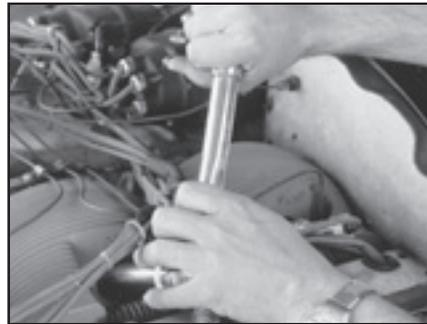
Tightening spark plugs with torque handle.
