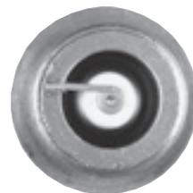
To equalize this wear, keep spark plugs in engine sets, placing them in trays identified by cylinder locations. After servicing the plugs, rotate as indicated in the following illustrations.
