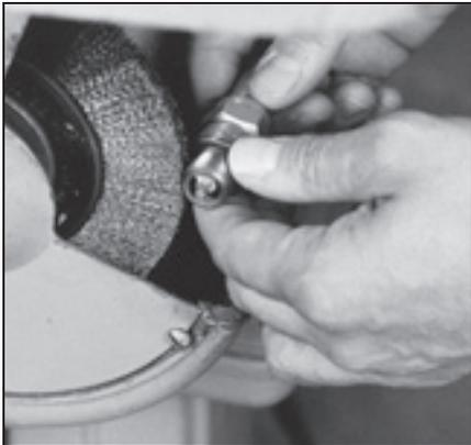
Cleaning threads with a rotary brush.
