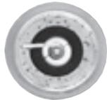
Ceramic in the firing end or shielding barrel chipped or cracked.
