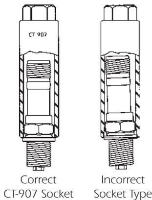
Correct CT-907 Socket      Incorrect Socket Type
