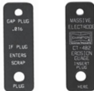
This gauge eliminates the guesswork in identifying a spark plug that should be replaced. It has been calibrated to allow insertion of properly gapped worn plug (see pg. 6).
