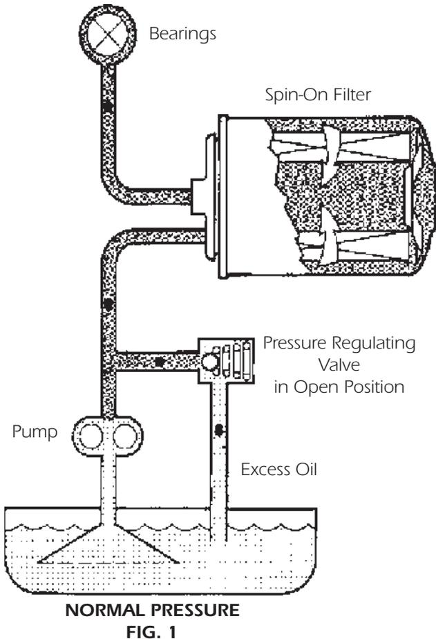
The oil pump supplies sufficient flow to lubricate the bearings and other moving parts of the engine. This oil must be under pressure if it is to properly separate the highly loaded parts of an engine and prevent excessive wear. The purpose of the regulating valve is to provide a constant pressure for the system.
