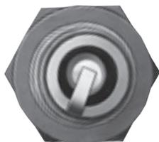
Single-Ground Electrode Automotive Gap Configuration
