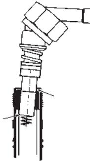
Connectors and spark plugs can be damaged by careless installation.
