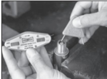
Setting gap on fine-wire spark plug.
