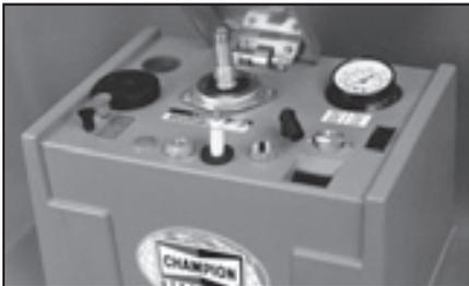
Cleaning firing end with model CT-475AV Cleaner/Tester.
