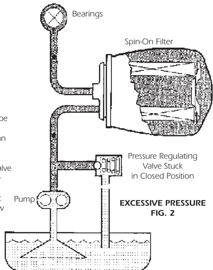
the point that many mechanics that are not familiar with lube systems fail to realize. Just remember any blockage in the system can also send the pressure beyond what the filter can stand which is rated at 400 psi. Burst.
