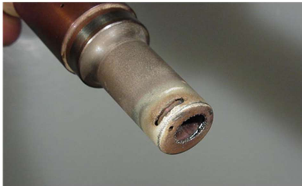
Figure 3: Unison Sidewall Erosion
