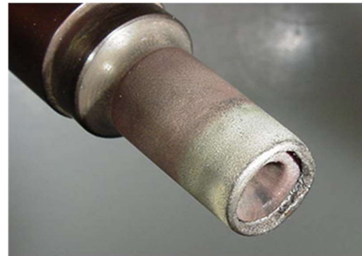
Figure 4: Unison Tip Loss from Sidewall Erosion
