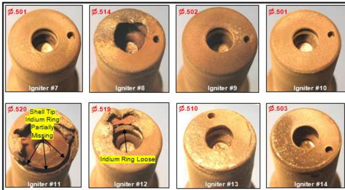
Figure 6. Unison Igniter Tips Exhibiting Severe Thermal Distress
