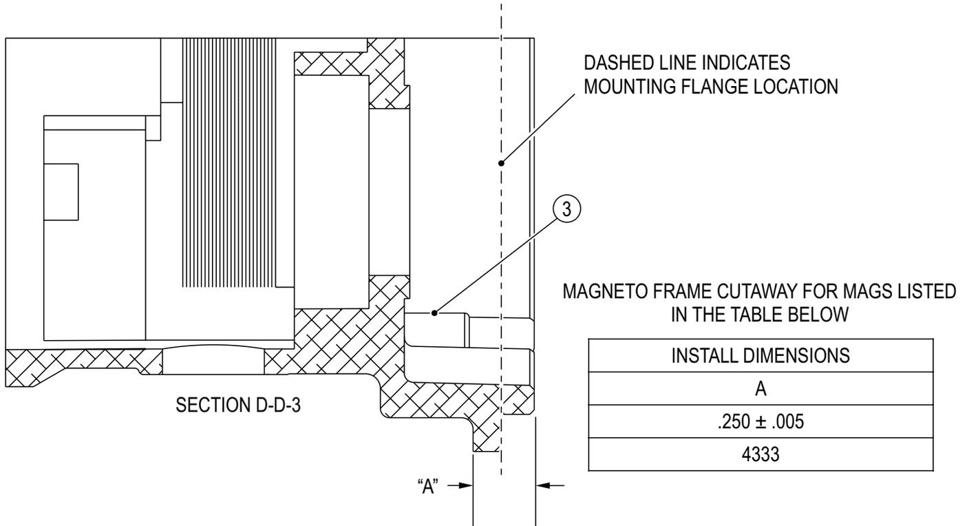
USE A CALIBRATED MEASURING DEVICE TO MEASURE DISTANCE "A", AS SHOWN IN CUTAWAY SECTION D-D-3. MAKE SURE THE FRAME SURFACE IS FREE OF CONTAMINANTS. ANY MEASUREMENT LESS THAN 0.245 INCH OF ANY PART OF THE STOP PIN (3), THE MAGNETO SHOULD BE REMOVED FROM SERVICE AND RETURNED TO CHAMPION FOR WARRANTY.
