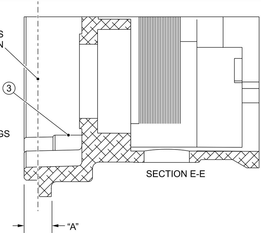
USE A CALIBRATED MEASURING DEVICE TO MEASURE DISTANCE "A", AS SHOWN IN CUTAWAY SECTION E-E. MAKE SURE THE FRAME SURFACE IS FREE OF CONTAMINANTS. ANY MEASUREMENT LESS THAN 0.432 INCH OF ANY PART OF THE STOP PIN (3), THE MAGNETO SHOULD BE REMOVED FROM SERVICE AND RETURNED TO CHAMPION FOR WARRANTY.
