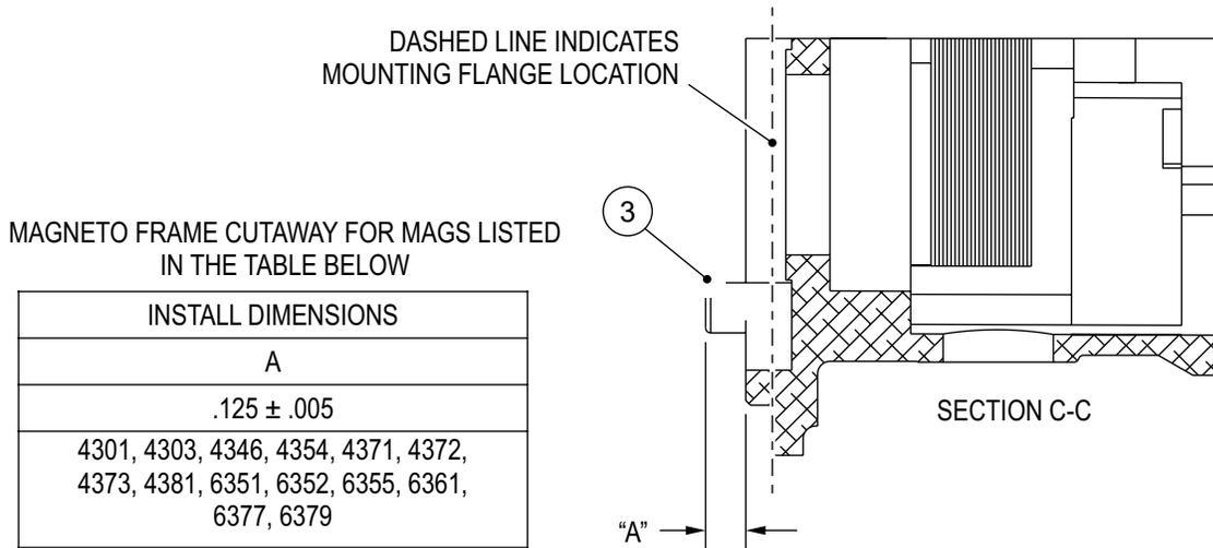
USE A CALIBRATED MEASURING DEVICE TO MEASURE DISTANCE "A", AS SHOWN IN CUTAWAY SECTIONS B-B AND C-C. MAKE SURE THE FRAME SURFACE IS FREE OF CONTAMINANTS. ANY MEASUREMENT GREATER THAN 0.130 INCH OF ANY PART OF THE STOP PIN (3), THE MAGNETO SHOULD BE REMOVED FROM SERVICE AND RETURNED TO CHAMPION FOR WARRANTY.
