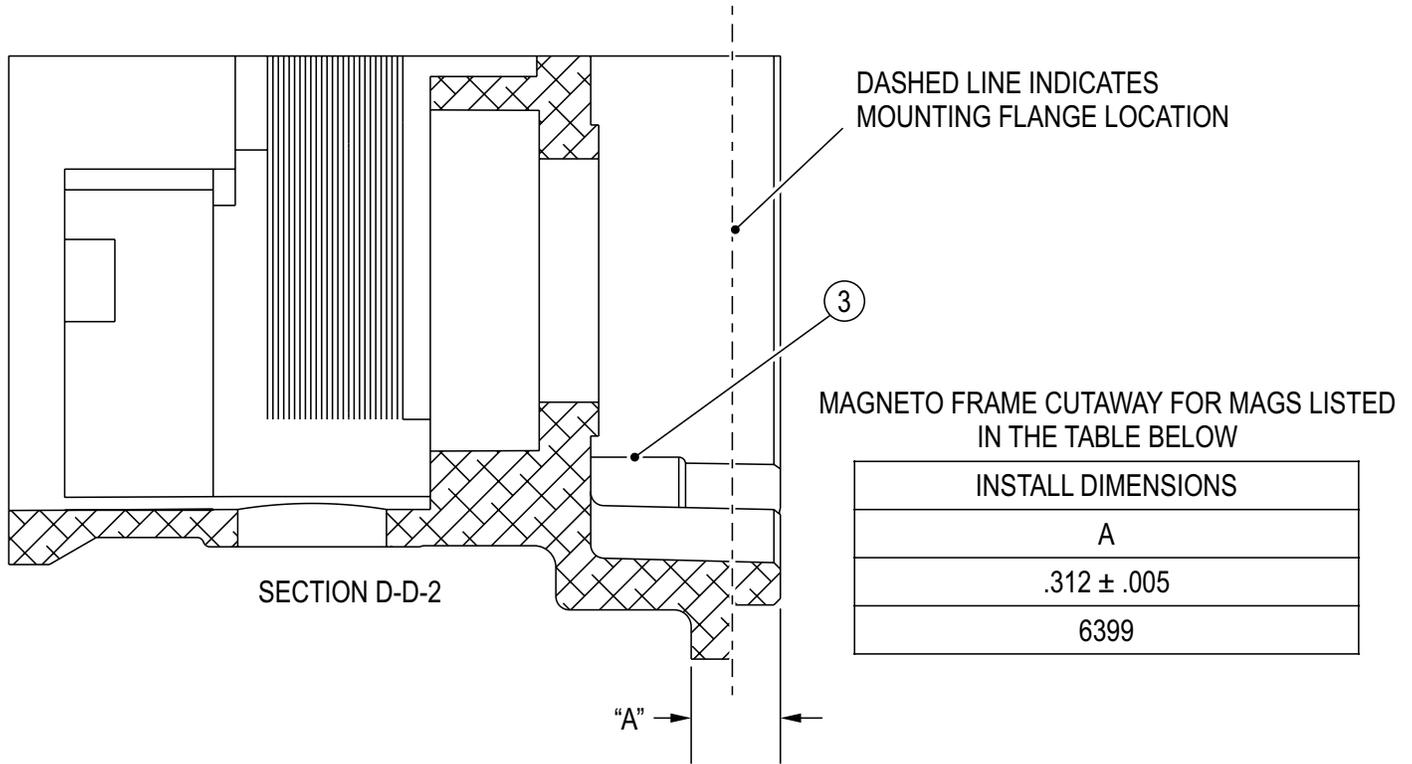
USE A CALIBRATED MEASURING DEVICE TO MEASURE DISTANCE "A", AS SHOWN IN CUTAWAY SECTION D-D-2. MAKE SURE THE FRAME SURFACE IS FREE OF CONTAMINANTS. ANY MEASUREMENT LESS THAN 0.307 INCH OF ANY PART OF THE STOP PIN (3), THE MAGNETO SHOULD BE REMOVED FROM SERVICE AND RETURNED TO CHAMPION FOR WARRANTY.
