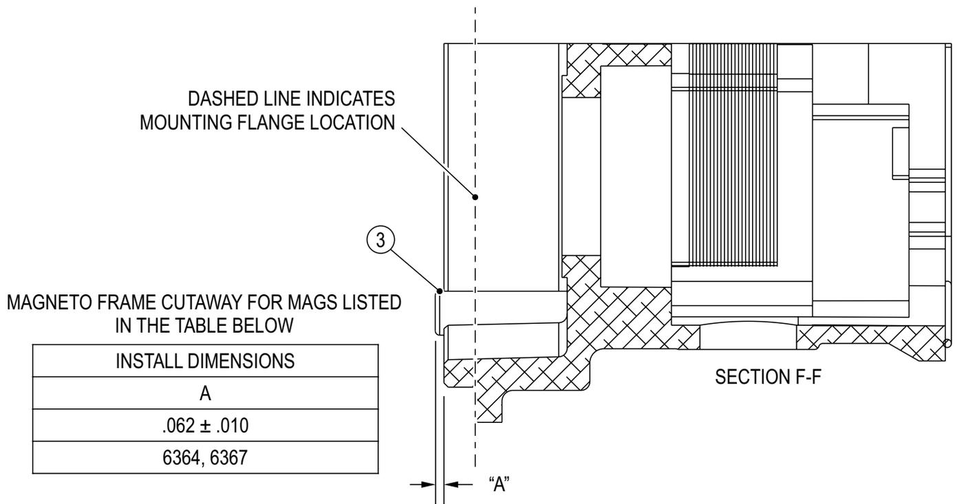
USE A CALIBRATED MEASURING DEVICE TO MEASURE DISTANCE "A", AS SHOWN IN CUTAWAY SECTION F-F. MAKE SURE THE FRAME SURFACE IS FREE OF CONTAMINANTS. ANY MEASUREMENT GREATER THAN .072 INCH OF ANY PART OF THE STOP PIN (3), THE MAGNETO SHOULD BE REMOVED FROM SERVICE AND RETURNED TO CHAMPION FOR WARRANTY.
