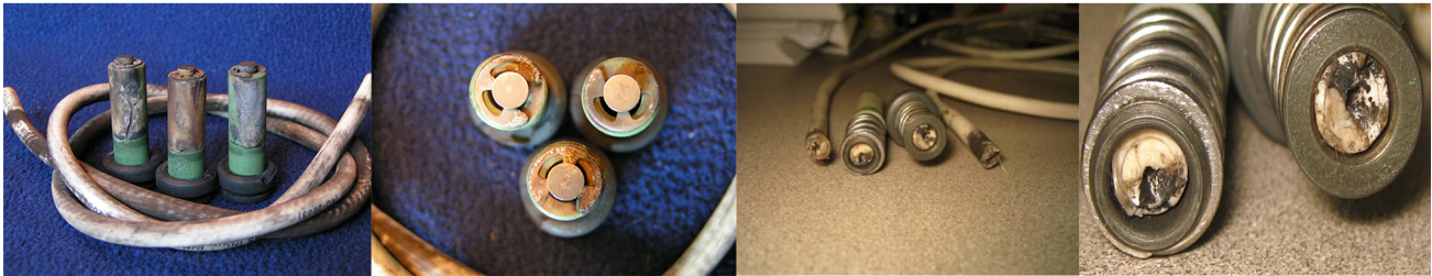
Original V2500 Ignition Lead Termination Design - (Non-Champion Parts) Figure 2
