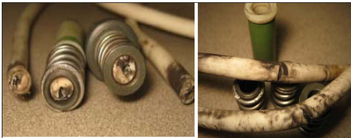
Figure 3. Photos of Competitive Lead with Severe Dielectric Failures in the Igniter Termination
