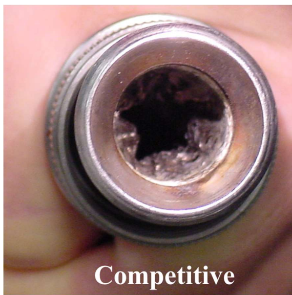
Figure 6. Comparison of Competitive (Collapsed) and Champion (Fully Open) Design Airflow Passage
