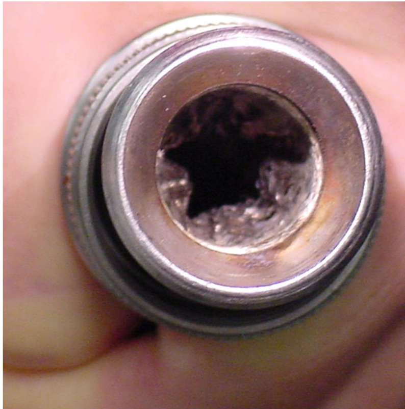
Figure 5. Photo of a Competitive Lead Design with Collapsed Innerbraid Resulting in Restricted Airflow
