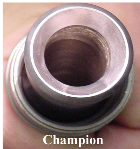
Figure 6. Comparison of Competitive (Collapsed) and Champion (Fully Open) Design Airflow Passage
