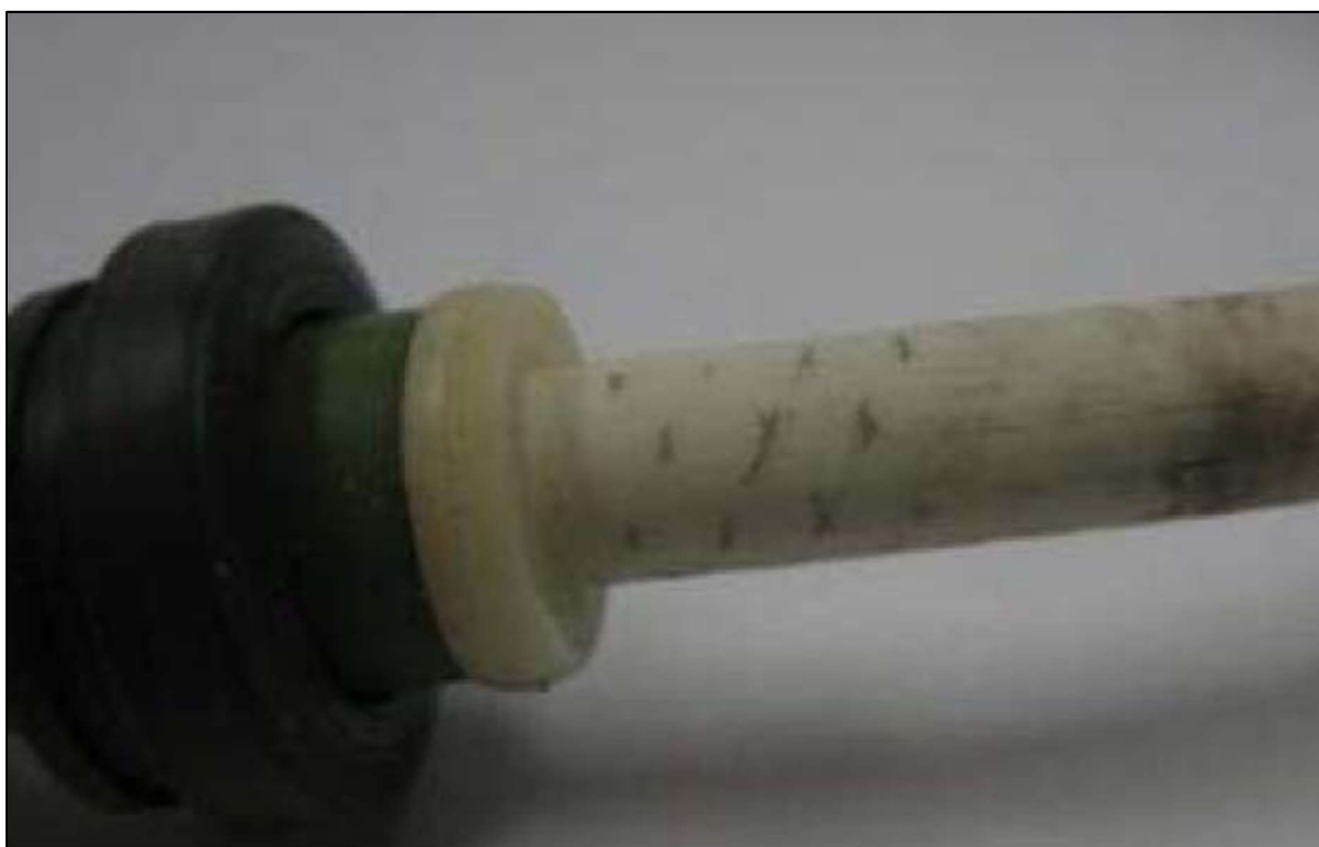
Figure 4. Photo of Competitive Lead with Corona Discharge Damage on Conductor Wire
