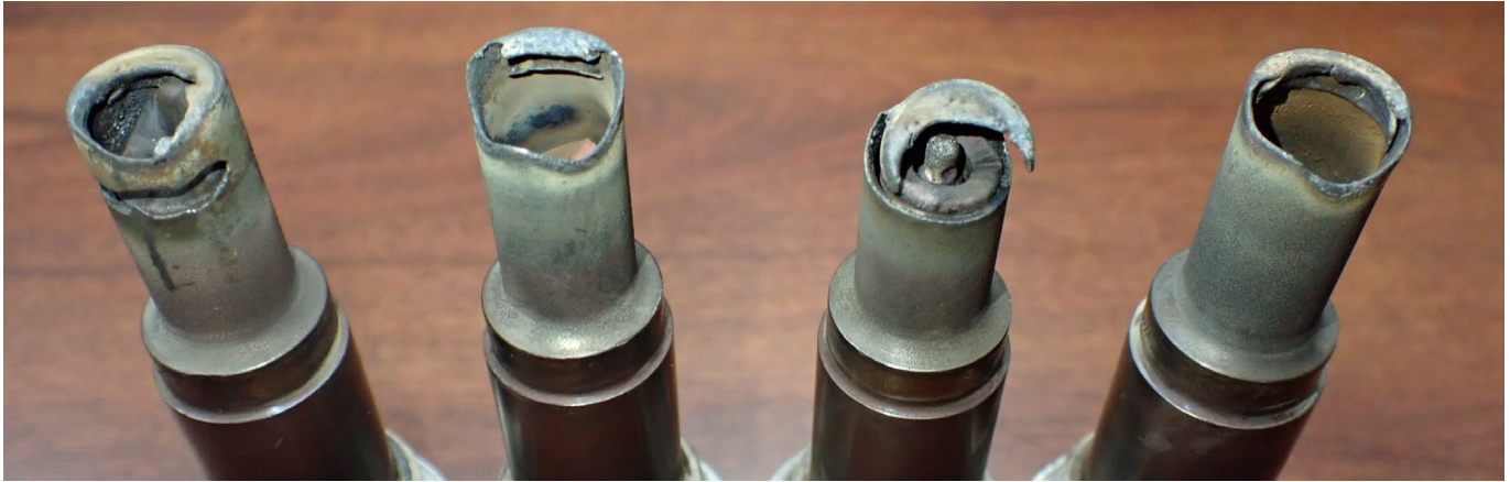
Figure 5: Igniters SN: LWY978, LYL040, LYA062, and LTY997. Total firing end deterioration with missing parts. See Figures 6-9 below.
