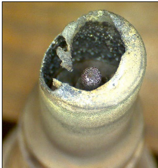
Figure 3: Excessive Shell Erosion
