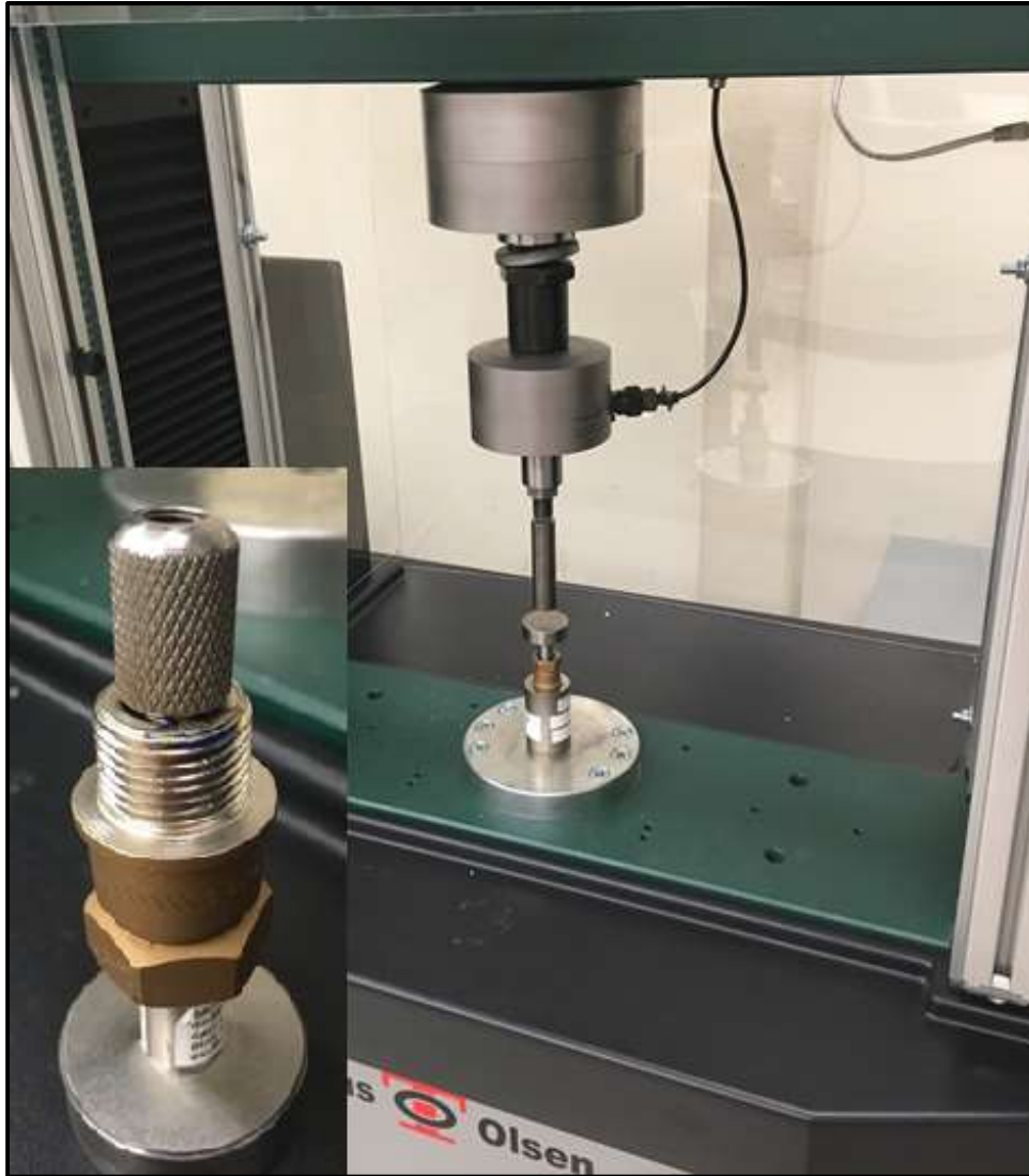
Figure 4: Pushout Test Setup
