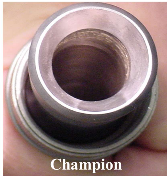
Figure 2. Comparison of Competitive (Collapsed) and Champion (Fully Open) Conduit Airflow Passage
