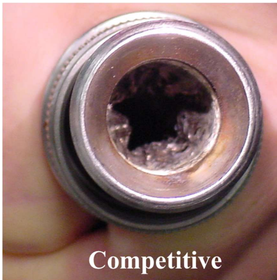
Figure 2. Comparison of Competitive (Collapsed) and Champion (Fully Open) Conduit Airflow Passage
