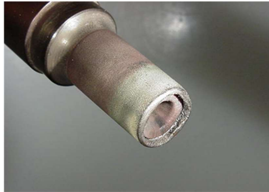
Figure 4: Unison Tip Loss from Sidewall Erosion
