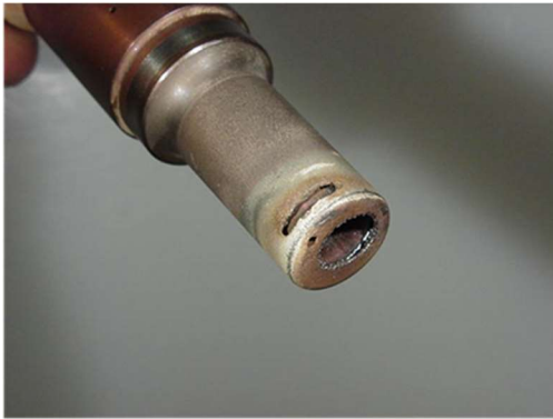
Figure 3: Unison Side Wall Erosion
