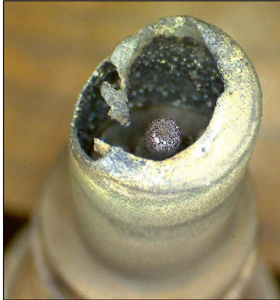
Figure 5: Excessive Shell Erosion
