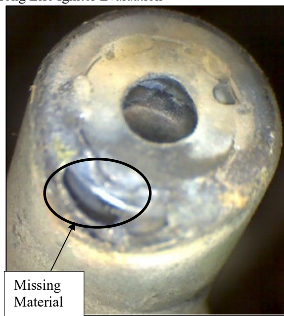
Figure 6: Firing End Shell Missing Material
