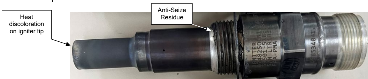
Figure 1: Typical Competitor Long Life Igniter Visual Examination
