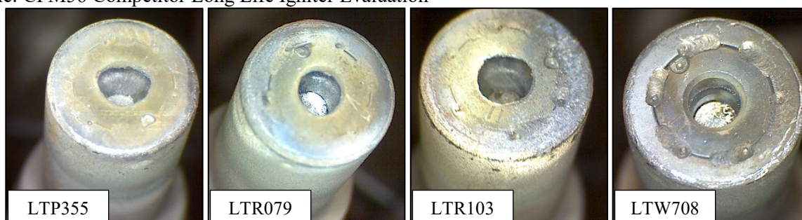
Figure 7: Competitor Long Life Firing Ends
